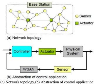
Fig. 1 WSAN Architecture without explicit controllers.
