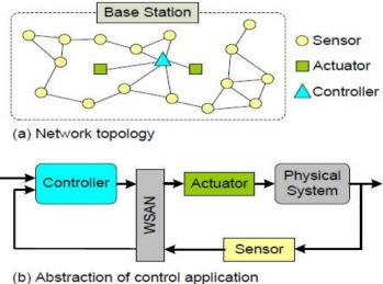
**Fig.2.** WSAN Architecture with explicit controllers.
